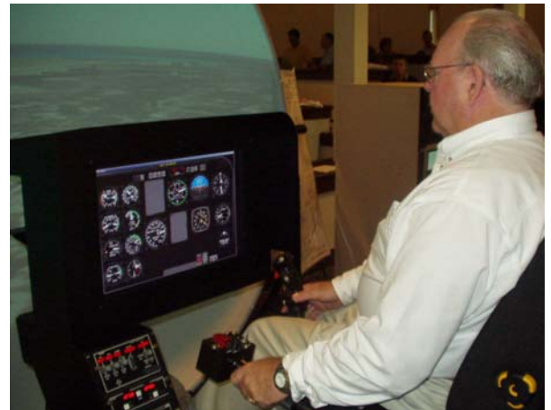
RealSims CEO Bob McGraw Demonstrates US ARMY TH67 Single Seat, Single PCIG Helicopter Procedures Trainer With Immersive 2.25 meter Hemispherical Dome Display and Low Cost Virtual Instrument Panel At US Army Research Lab Ft Rucker Alabama
